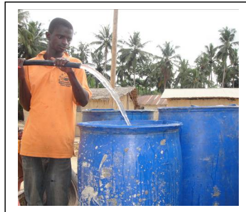
Figure 16. Discharge during development 35 litres/minute
