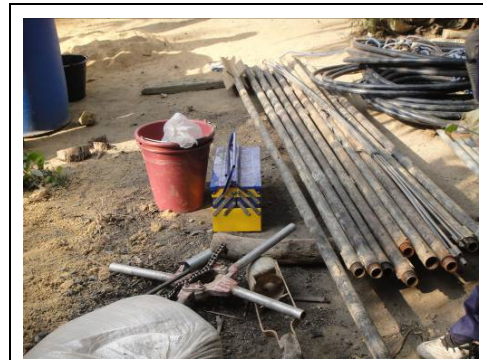
Figure 8. Drilling tools for rotary jetting
