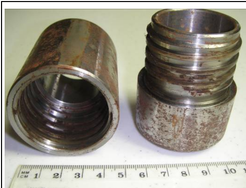
Figure 3. Coupling for drilling rod (50 mm)
